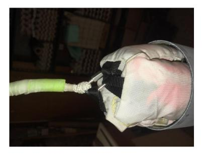
8) The quick-link from the drogue and NC connected to the loops of the d-bags AND the TD-2. Note that while I do want significant force holding the d-bags to the TD-2 (So they will NOT fall out!) I still needed to use an additional quick-link as a spacer.
