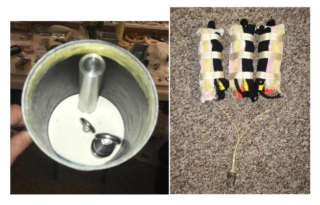
5) The quick-link for the 3 mains, is connected to the center eyebolt.
