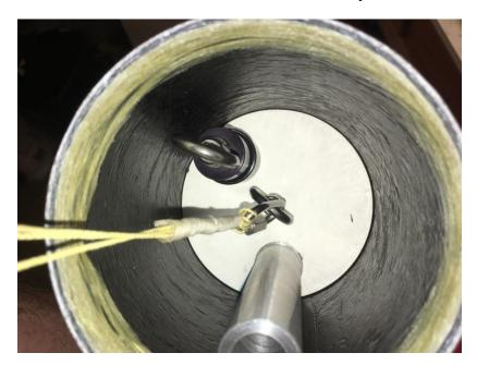
6) The 3 mains are tucked into the coupler. Note the gas conduit is not obstructed.
