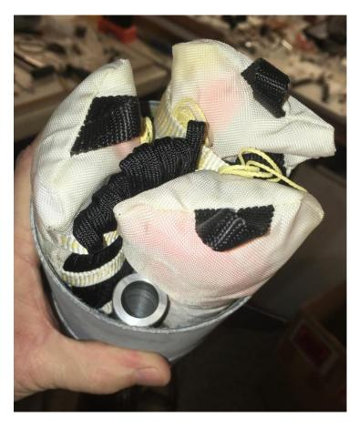
7) The quick-link from the drogue and NC (Not shown) connected to all 3 of the loops on the top of the main d-bags.
